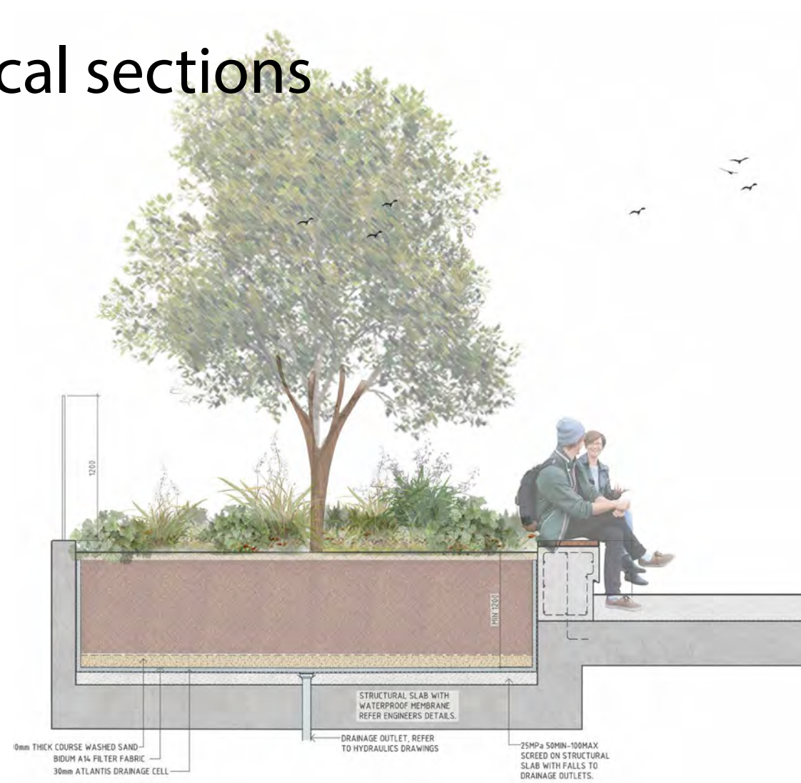
01 PLANTER ON STRUCTURE WITH SLAB SET(DOWN AND SEATING
