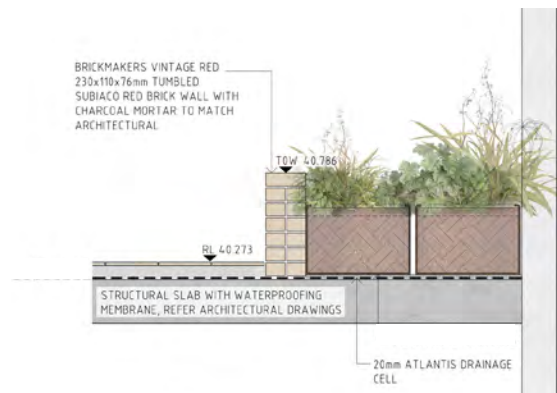
03 MASONRY WALL WITH HDPE PLANTER INSERTS
