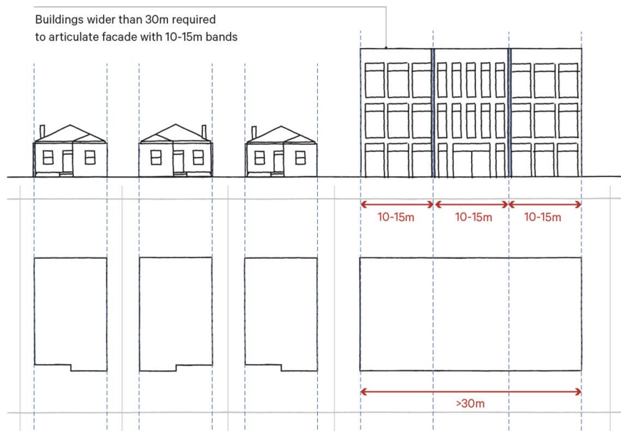
Figure 5. Vertical articulation of buildings wider than 30m
