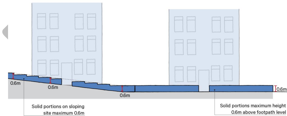
Figure 7. Walls within the street setback area
