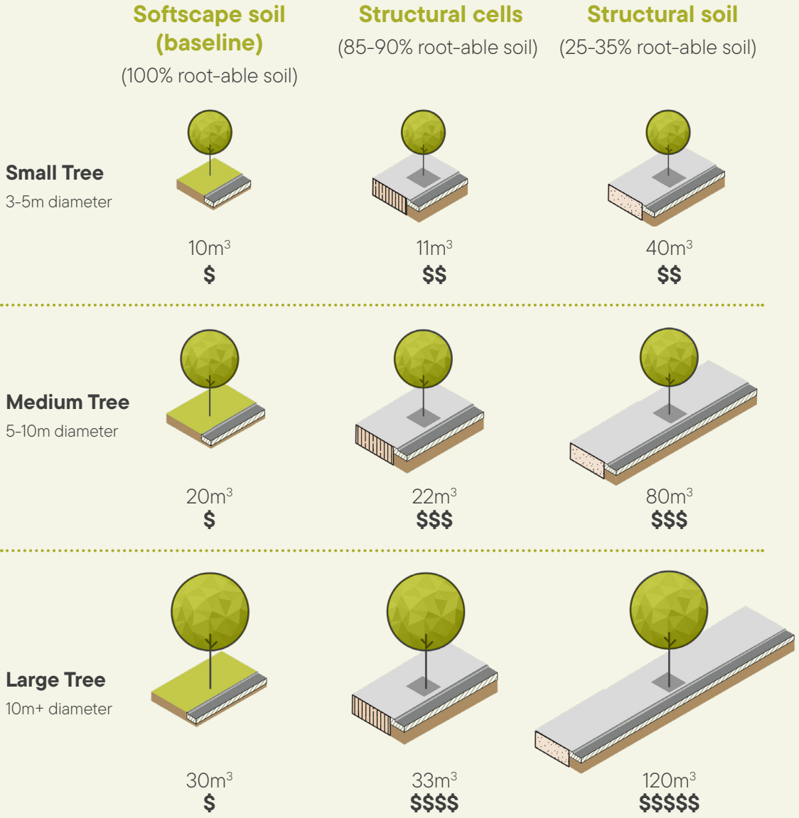
Figure 15: Space requirement and cost comparison of structural cells and soils
