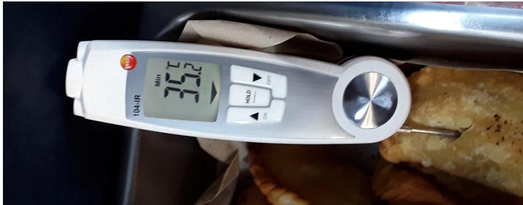
Figure 5: A probe thermometer demonstrating that food is stored at a temperature within the danger zone.
