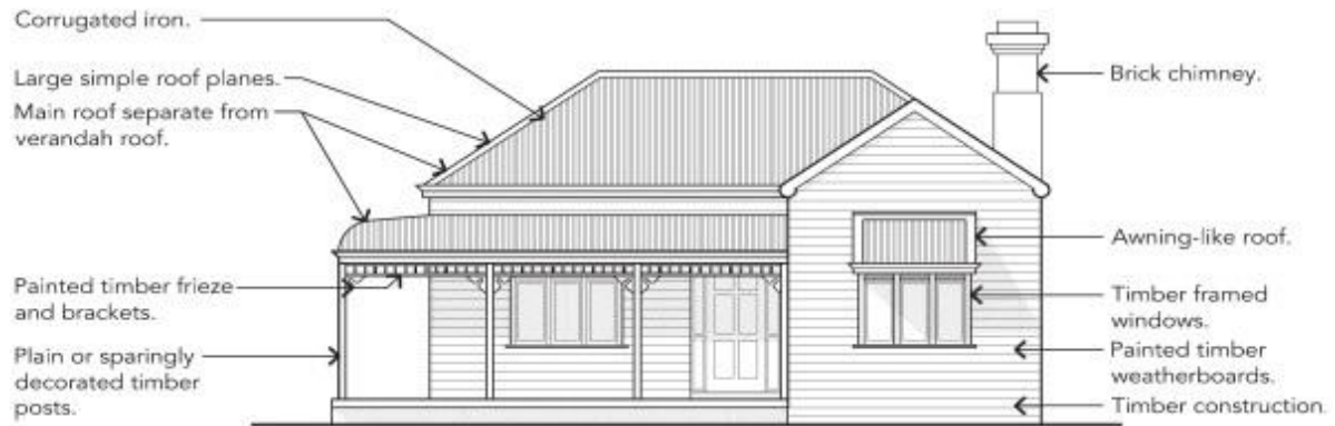
Primary Elevation - Example of a Federation Timber Bungalow
