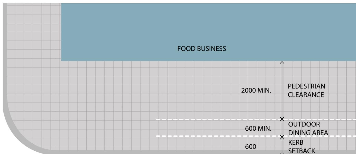
\*Pedestrian Clearance determined by Figure 2: Pedestrian Clearances
