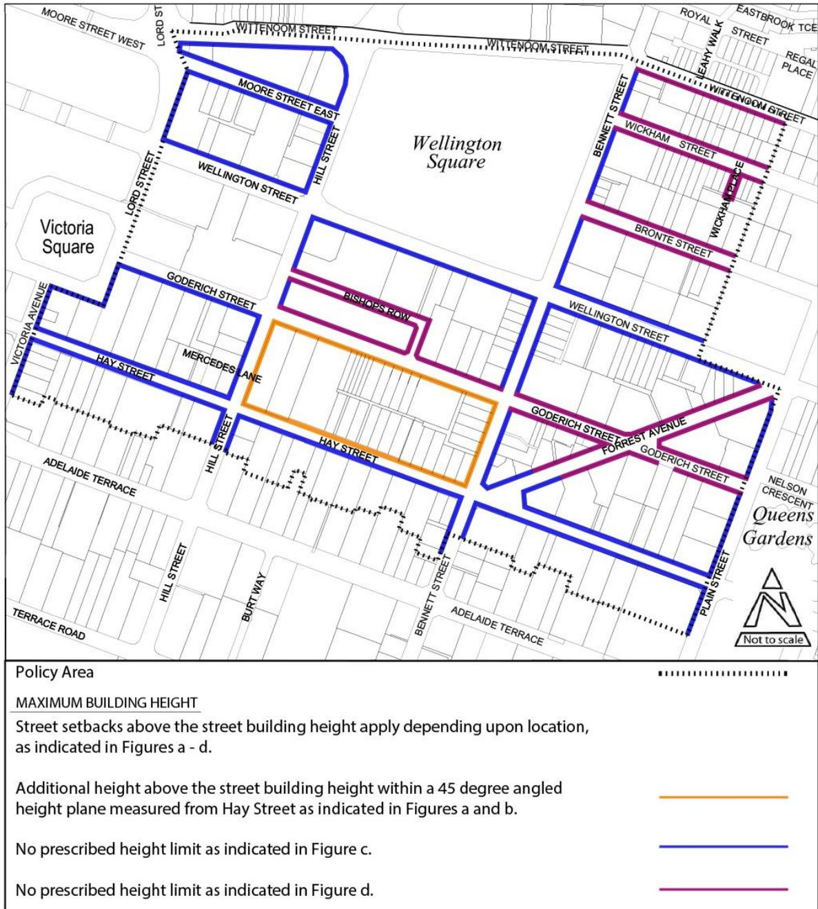
Figure 3 – Goderich Design Policy – Maximum Building Height Plan (1 of 2)
